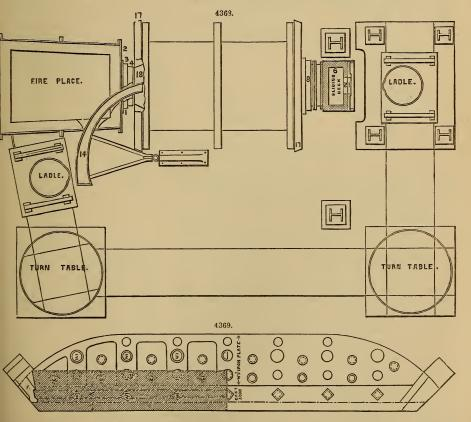
proportionate to the capacity of the revolving chamber. The bridge is a common water-bridge, open on the top and bolted on the end plate of the furnace. The bridge neck has a flange or ring upon it, for the double purpose of confining the brickwork immediately above the bridge, and for supporting a loose ring which serves to form a close joint between the fire-grate and the revolving chamber. The revolving chamber is a long square box, as in the centre of the machine just 6 s
